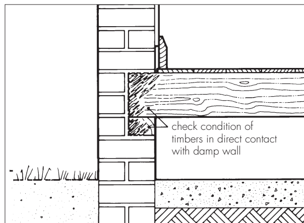
Figure 2 Check embedded timber for decay
